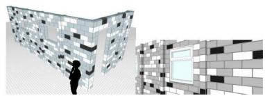
Figure 3. The Everblocks modular building blocks used to create the reconfigurable space.
